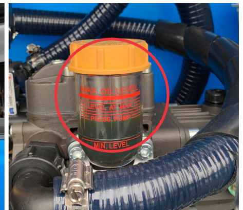
Pump Sight Glass. Check oil level on pump when running. (Oil should not exceed max line)
