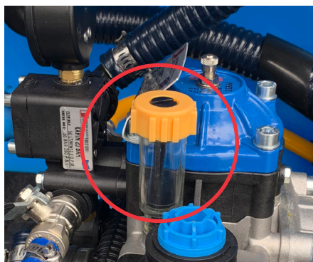
Pump Sight Glass (Oil should not be seen in sight glass when the pump is off)
