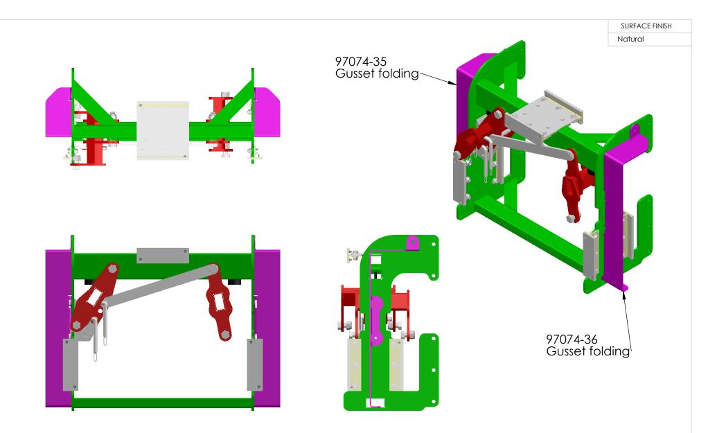
The 18M boom assembly requires these two extra bolt on components
