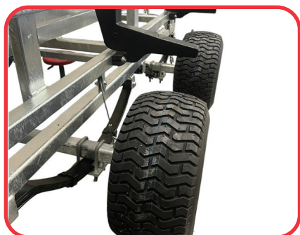
High load carrying in tandem axle design.
