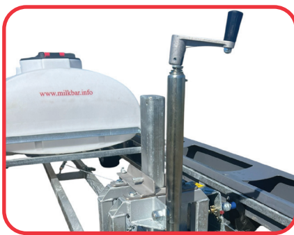
Front to back and sideways levelling system.
