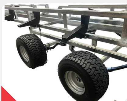
Pull wires used to compress springs to achieve sideways levelling.
