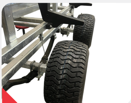
High load carrying in tandem axle design.
