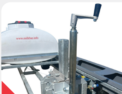
Front to back and sideways levelling system.
