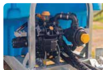
HYDRAULICALLY DRIVEN DIAPHRAGM PUMP
