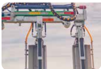
HYDRAULIC ROW ADJUSTMENT (2.4–3 Metres)
