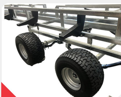
Pull wires used to compress springs to achieve sideways levelling.
