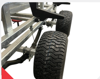
High load carrying in tandem axle design.
