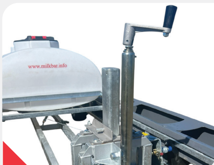
Front to back and sideways levelling system.
