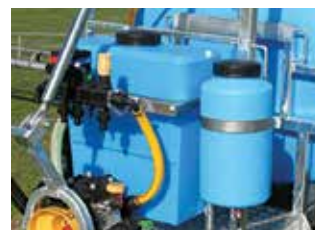
FLUSH & HANDWASH TANKS
