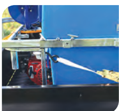
COMPACT WRAP AROUND HEAVY FRAME WITH INTERGRATED TIE-DOWN POINTS
