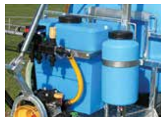
FLUSH & HANDWASH TANKS
