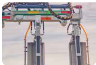
HYDRAULIC ROW ADJUSTMENT (2.4–3 Metres)
