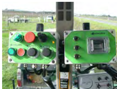
Three operating modes to open and to close the head of the Pre-Pruner
