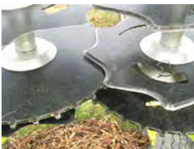
Cutting blade and notched discs = efficient clean cuts and trellis post protection
