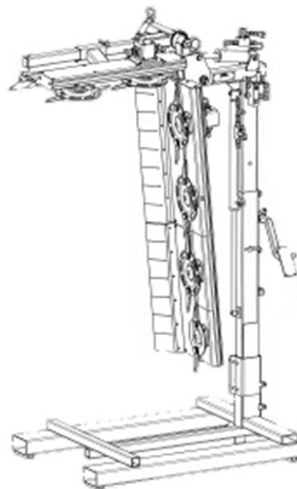
Drawing shown with optional 4th Vertical blade.
