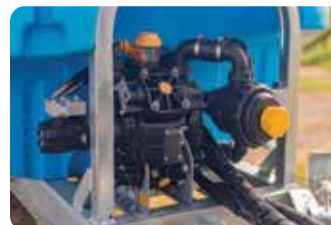
HYDRAULICALLY DRIVEN DIAPHRAGM PUMP
