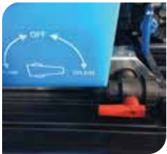
3-WAY DRAIN TAP: PUMP, OFF AND DRAIN
