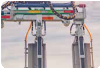
HYDRAULIC ROW ADJUSTMENT (2.4–3 Metres)
